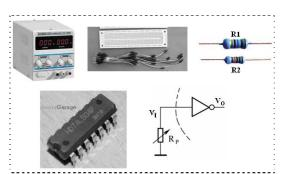
Figure 3. Devices and test circuit used in load characteristic experiment
