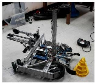
Figure 5. Robot with Pixy camera
