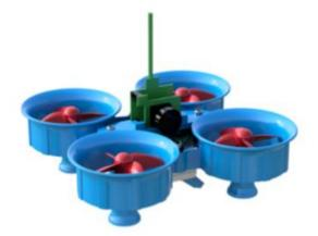
Figure 1. Assembled 3D model of a Micro Drone (Autodesk Design Academy, 2018)
