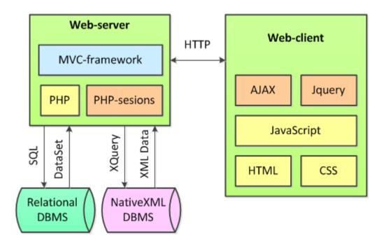
Figure 3. Typical architecture of web-based information system developed by a student
