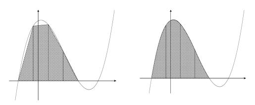
Figure 2. Trapezoidal formulas (left) and Simpson methods (right)
