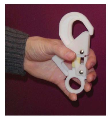
Figure 1: Prototype Safety Hook from Pensafe Project, produced by an RPM
