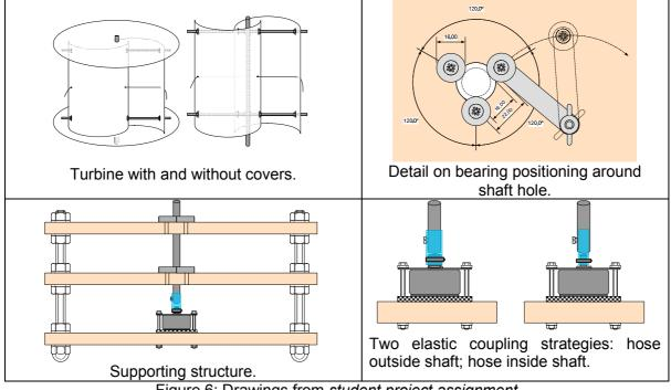
Figure 6: Drawings from student project assignment
